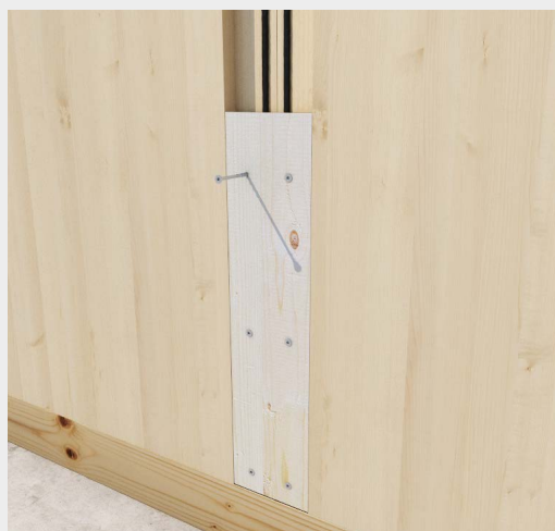
Fastening CLT walls with 6 mm diameter HBS screws.
